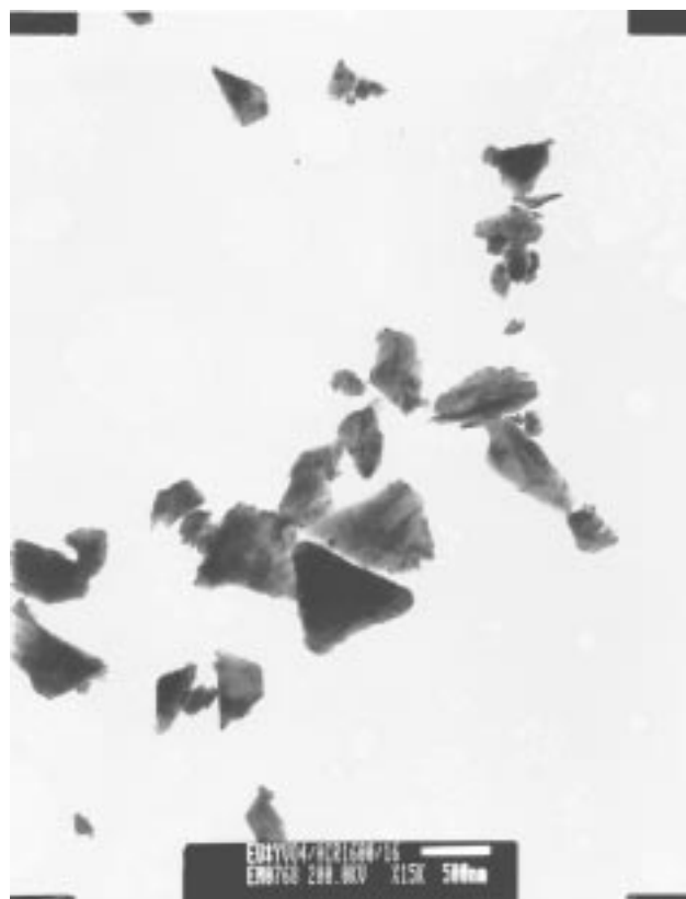
Fig. 7 TEM micrograph of stoichiometric Eu^{3+}:YVO_4 powder reacted by the HCR technique after firing at 1600^\circ C for 16 hours. This powder has very high emission peak (6537 arb. units) at 619 nm compared to Sylvania 2391 standard (6881 arb. units).
